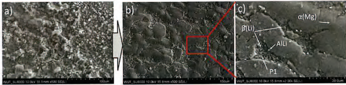
Fig. 11. Characterization of corroded surfaces of the conventionally extruded Mg-7.5Li-3Al-Zn alloy after 1 h of immersion in 0.01 M NaCl: a) surface covered with corrosion products, b) surface without corrosion products, c) surface without corrosion products shown at higher magnification.
