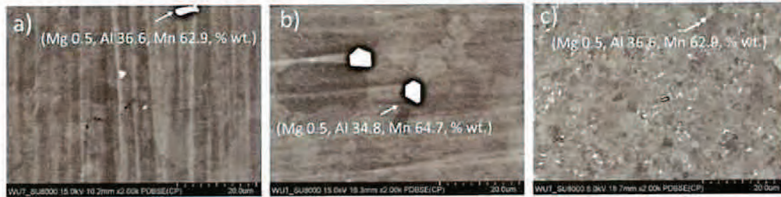
Fig. 4 – SEM microstructure images of AZ31 alloys extruded to: a) Ø6 mm, b) Ø4 mm, and c) Ø2 mm.
