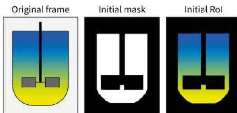
Figure 6. An example of initial region of interest selection. A binary mask is constructed, which excludes the elements of a frame, which interfere with the observation of vessel contents. The mask is overlaid on top of the original frame to obtain an image for further processing.
