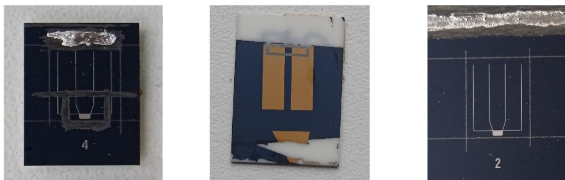
Figure 8.1 Photographs of devices on \text{ZrO}_2 used in this study. Left – solar cell used for DLCP measurement, with active surface reduced through mechanical scribing. Middle – thin film used for conductivity measurements, with measured area defined by mechanical scribing (rectangle in the top of the device). Right – 50\text{mm}^2 solar cell used for STC JV measurements by ZSW.
