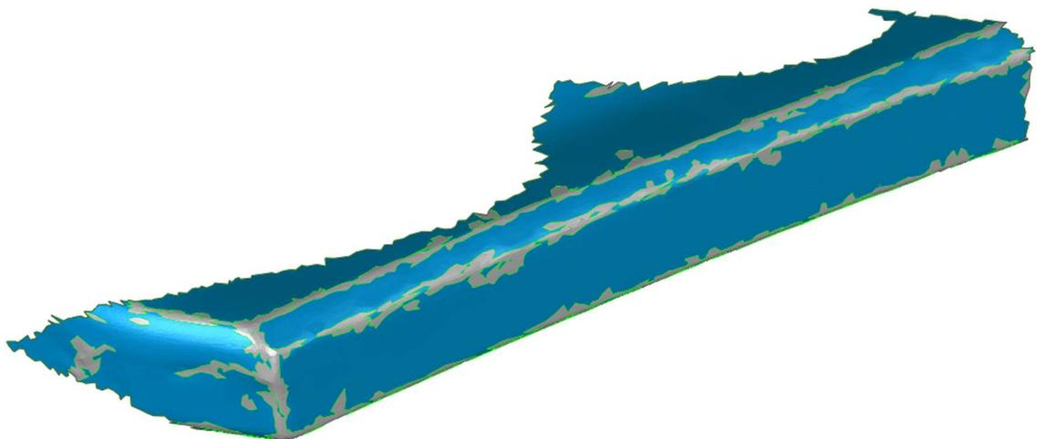
Fig.5.19. De-featured example for a surface flatness inspection[38].
