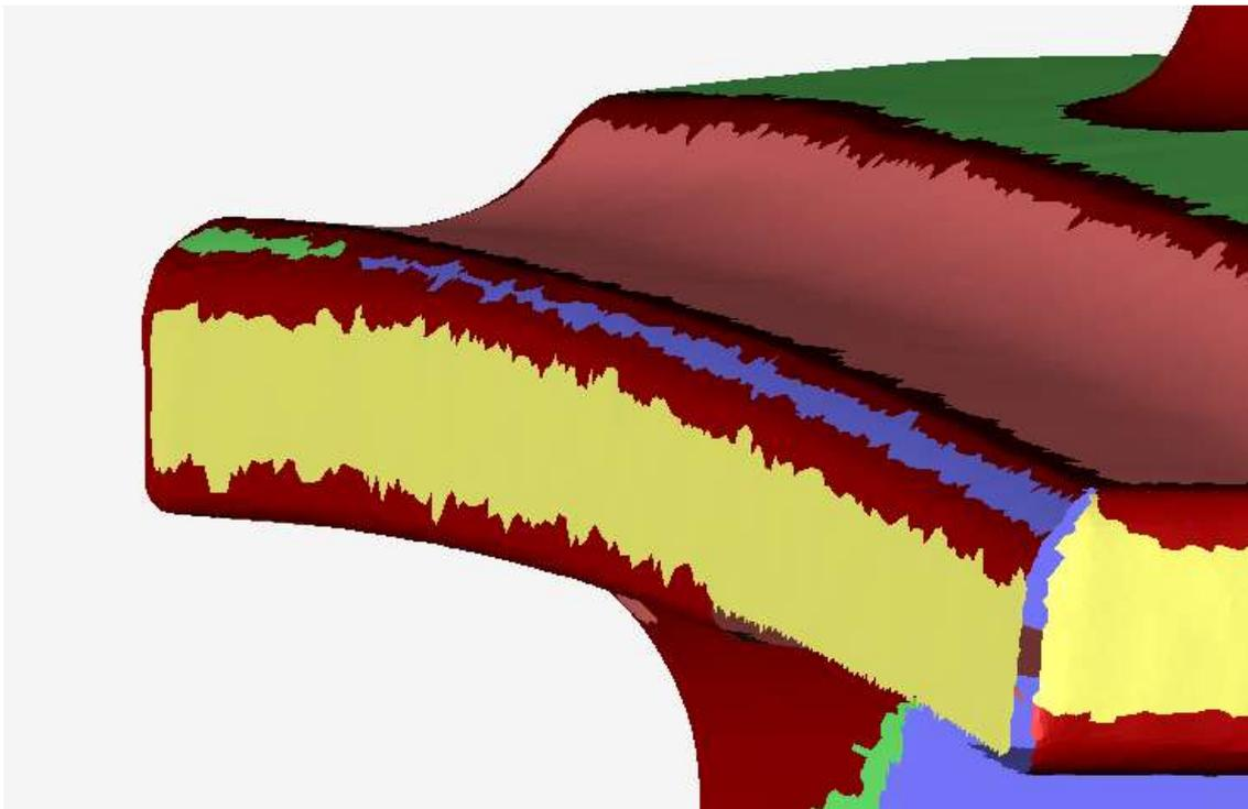
*Fig.5.11. Surfaces identified on a 3D raw scan with small contours to be deleted from the file[38].*
