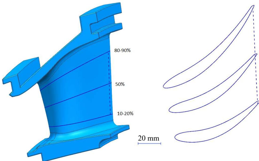
*Fig.5.1. Turbine guide vane CAD Model with original CAD sections used for airfoil extraction with additional trend line. [39]*
