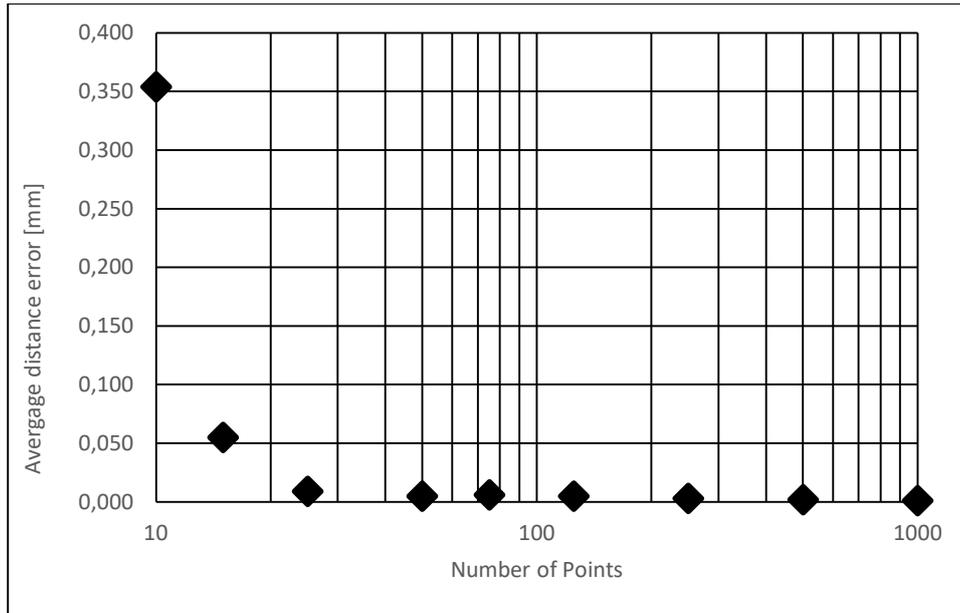
Fig.5.5. Distance error chart for the set of points in the range of 10-1000. [39]
