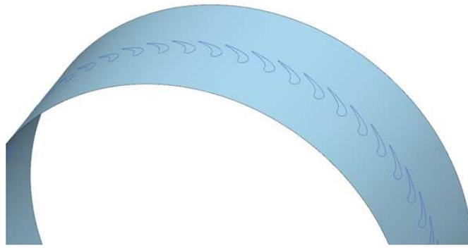
*Fig.1.3. A 3D section through the set of turbine guide airfoils.*
