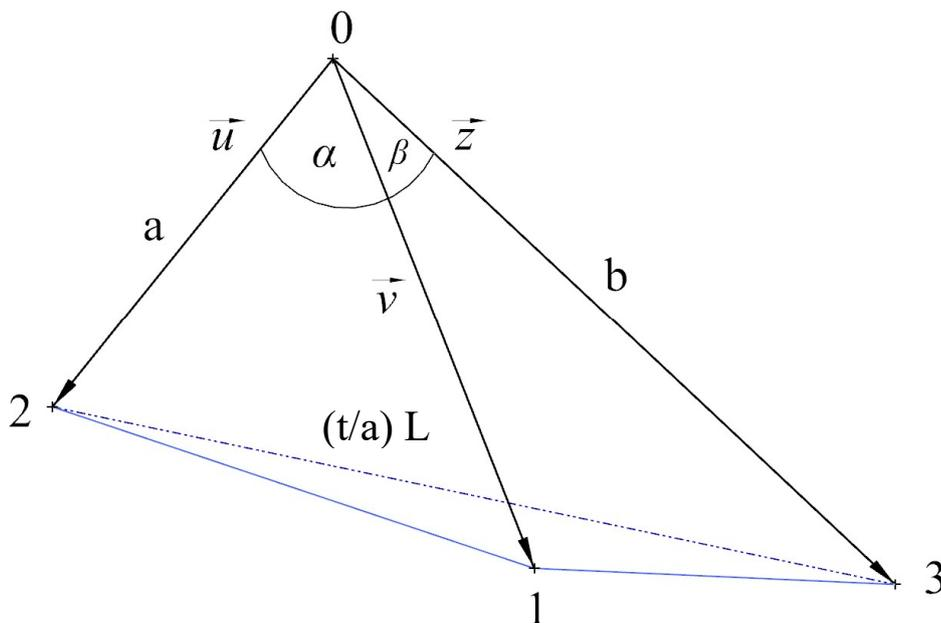
Fig.5.15. A pair of triangles. aL is the 3D distance, while tL is the theoretical value which can be calculated using trigonometrical equations[38].
