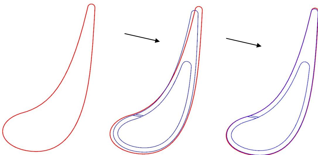
Fig.3.2. An example of 2D airfoil section process loop: A) Hot external aero shape (red), B) Cold scaled shape with engineering constraints and variables C) FEM iteration to utilize engineering variables to match original input shape in hot condition.
