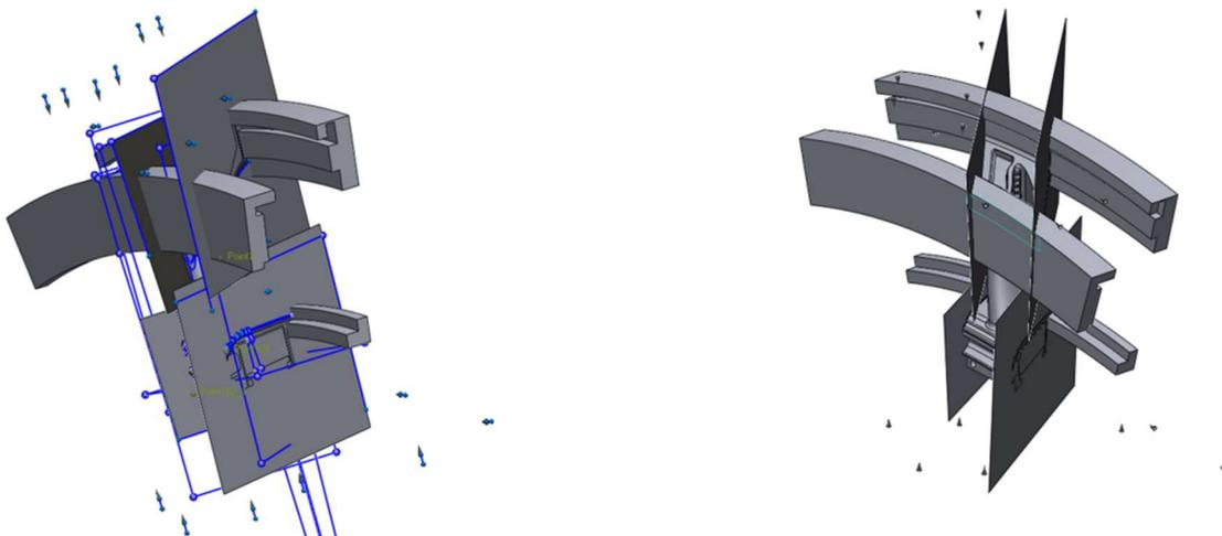
*Fig.1.14. Example of a CAD File imported to another system. a) total data, b) solids and surfaces only*
