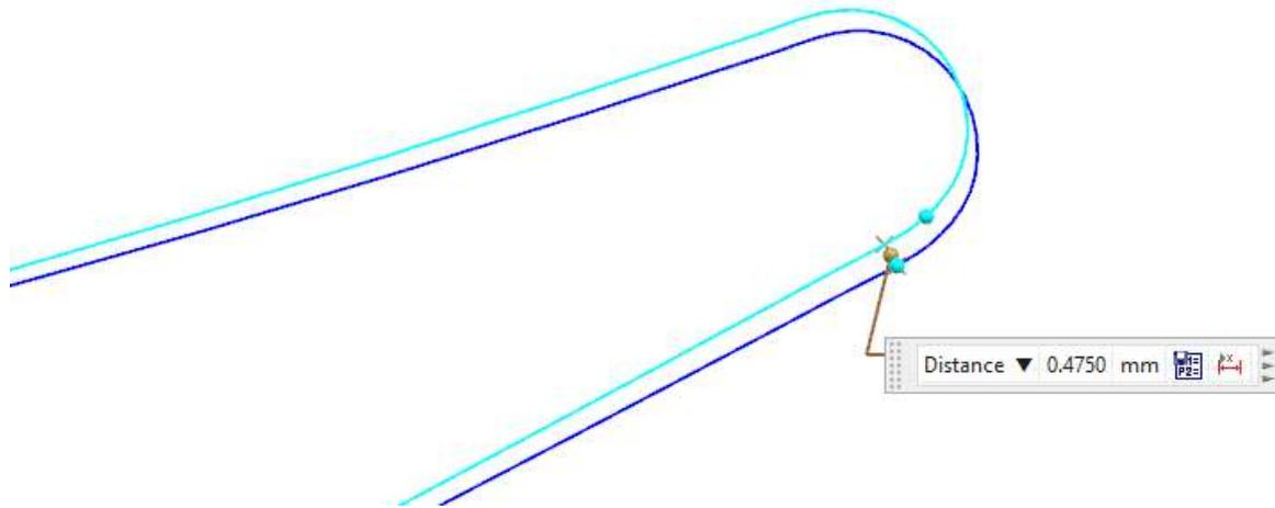
Fig.3.4. Trailing edge validation: from a hot external shape to add details on cold deformed shape and back into hot condition shape for comparison.
