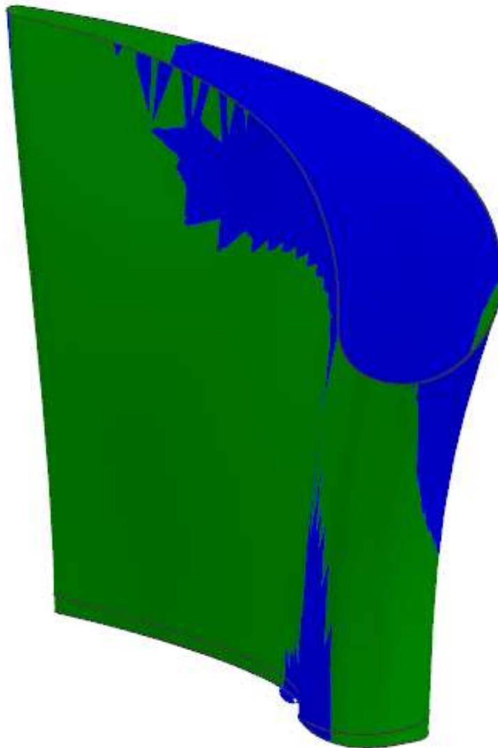
Fig.3.6. Overlay of the cold shapes based on Powell and Conjugate Gradient deformation loop.
