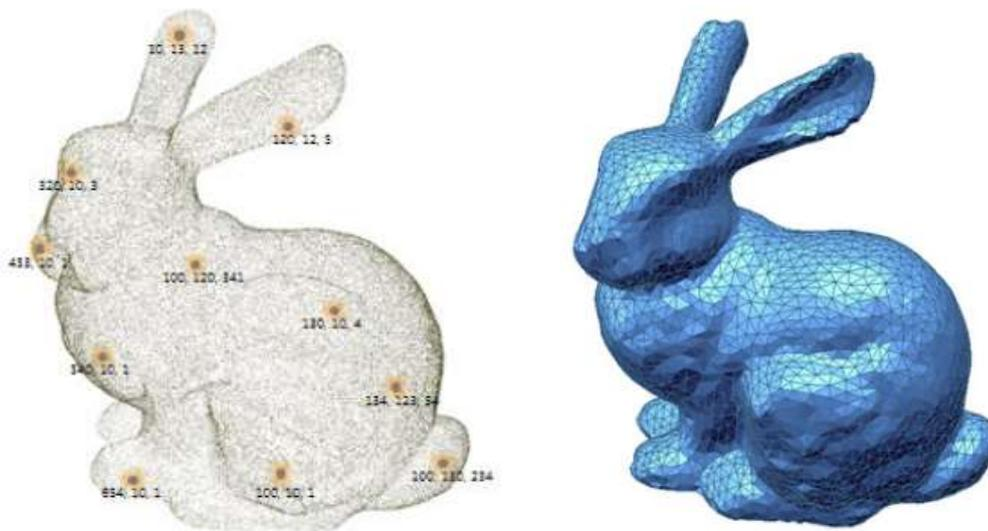
*Fig.1.24. Point cloud on the left and triangulated mesh surface on the right [98]*
