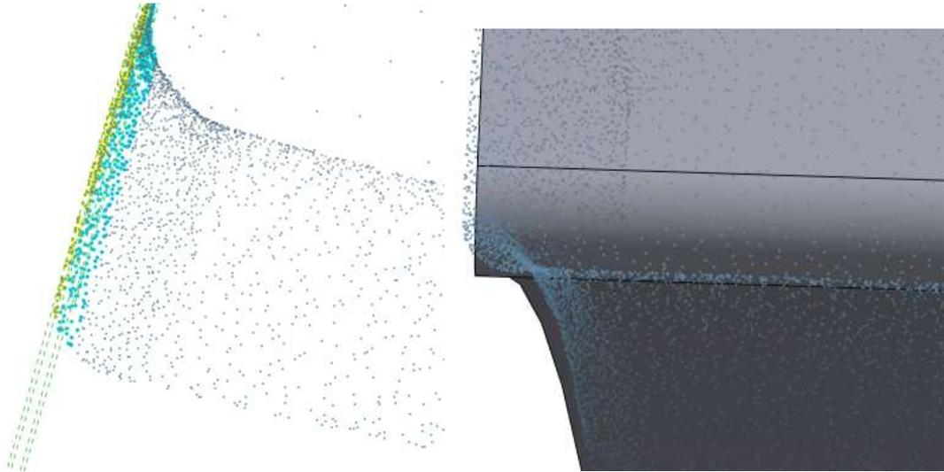
*Fig.5.10. Geomagic Control X inspection. Some of the points used for a flatness inspection come from a “blend” area, not introduced on a CAD model[38].*
