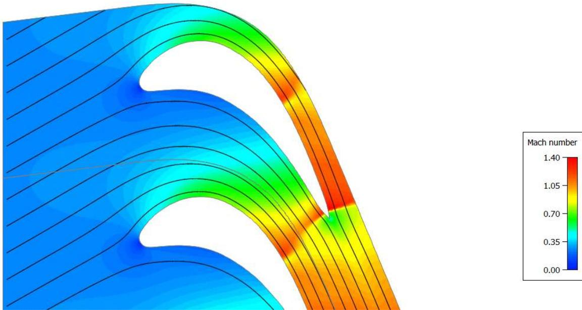
*Fig.1.13. Throat impact on the local flow change (example)[42].*
