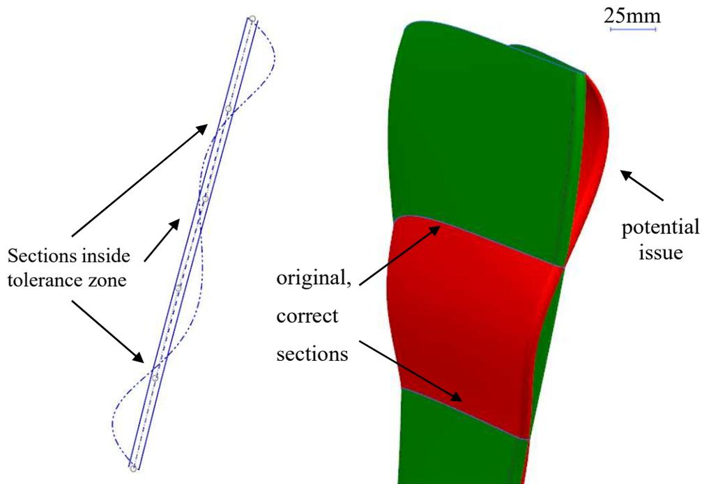
*Fig.5.3. An exaggerated example of a potential miss during the inspection process. 2D sections measured separately can be within tolerance, while the overall airfoil shape may be bent/curved[39].*
