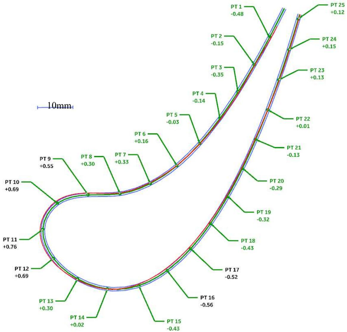
Fig.5.8. CMM inspection results for a turbine guide vane section with 25 significant points [mm][39].
