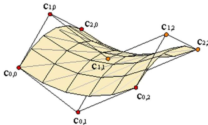
Fig.1.7. B-Spline surface example [100]
