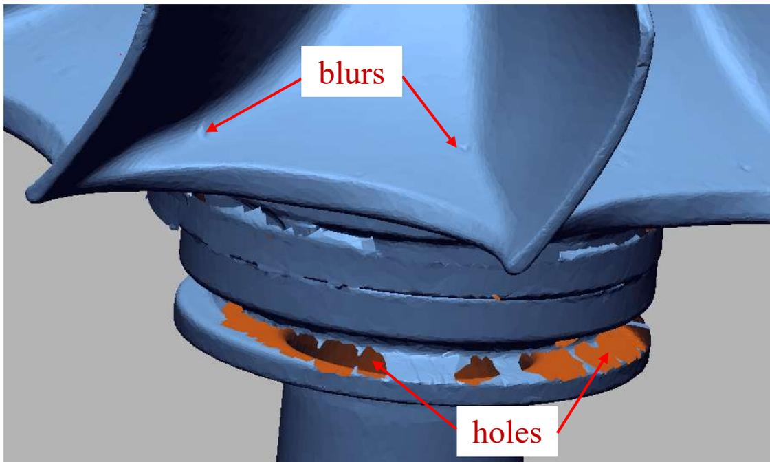
*Fig.1.23. Blurs and holes are typical imperfections of 3D scans [98].*
