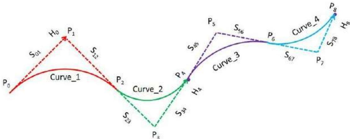
Fig.1.6. B-Spline curve example [73]
