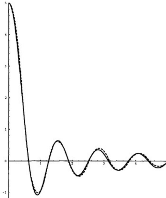
*Fig.1.22. An example of the spline with 999 knots (solid line) and simplified one after removing 986 of them (dotted) [69]*
