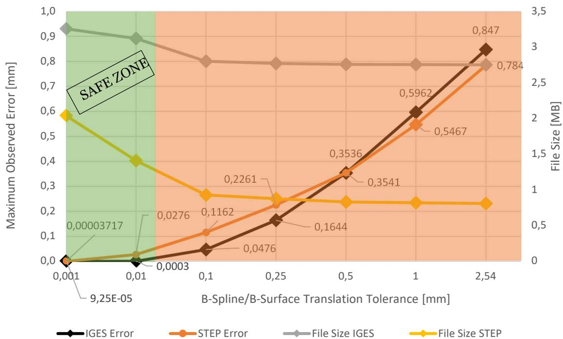
Fig.4.5. An average surface error vs. the original shape with a comparison of tolerance and file size.
