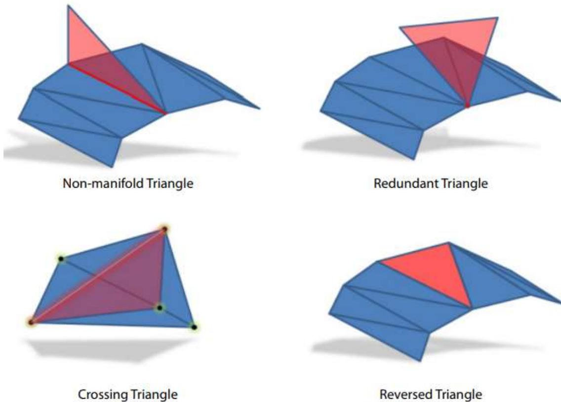
*Fig.1.26. Examples of mesh flaws[98]*
