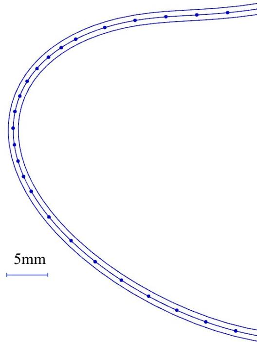
*Fig.5.2. Airfoil 2D section with visualization of GD&T tolerance zone[39]*
