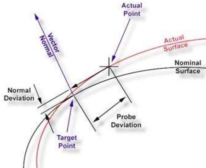
*Fig.1.21. The actual surface may differ from the original CAD shape[103]*
