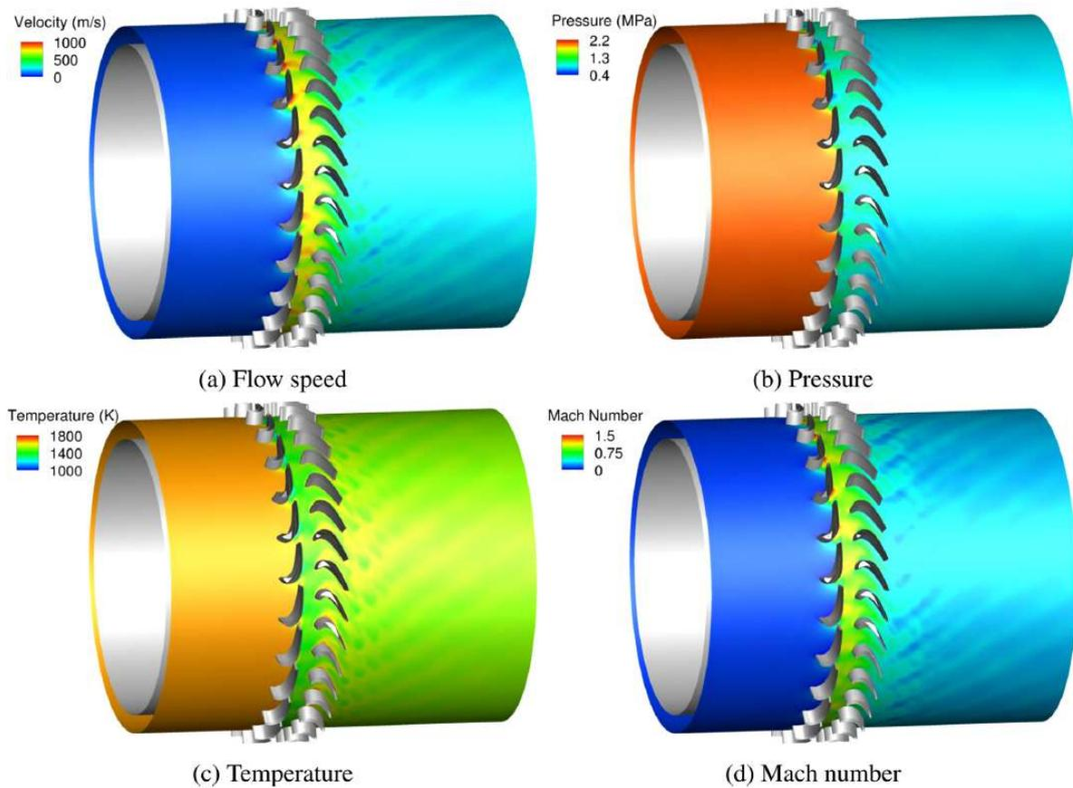
*Fig.1.2. Flow variables inside a gas turbine[80].*
