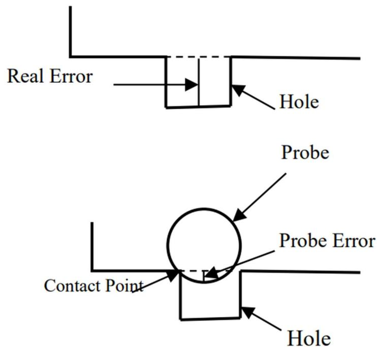
*Fig.1.20. Real “small” surface issues will not be measured by CMM correctly. This kind of issue will be identified under NDT methods like FPI or DPI.[4]*
