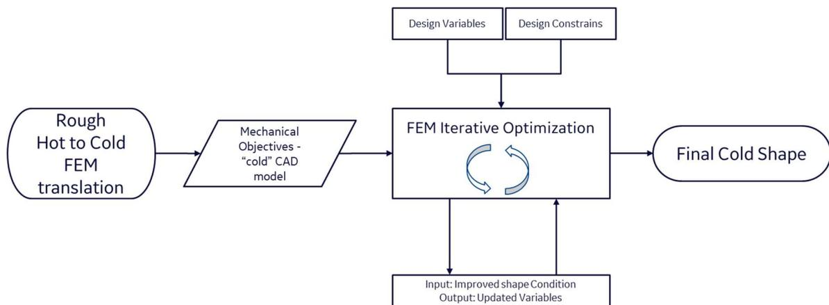
Fig.3.1. An iterative loop for the prototyping cycle.
