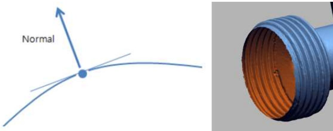
*Fig.1.25. Additional normal vector helps to visualize the entire model in the computer system. Blue color for external surface and orange for internal [98]*
