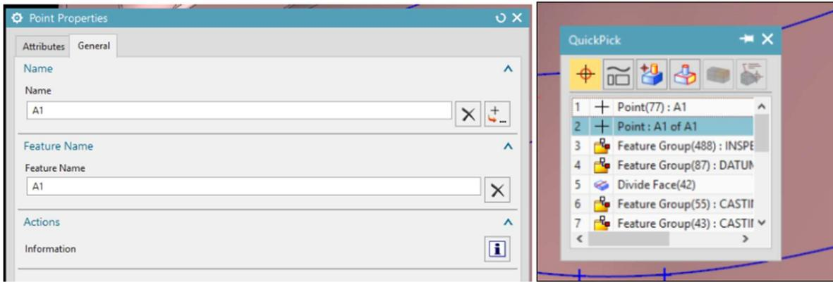
Fig.4.1. Point name and feature name comparison: The feature name is internal, the name is internal and external, and can be exported to a neutral format file.
