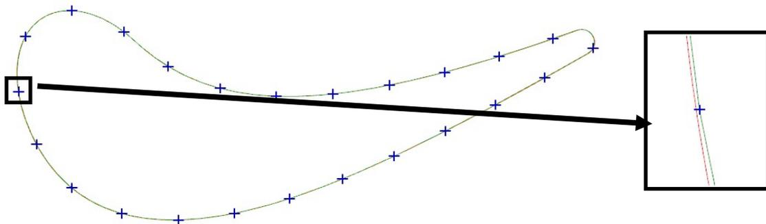
Fig.3.8. Twenty-four representative points overlaid with on the original - initial hot CAD section.
