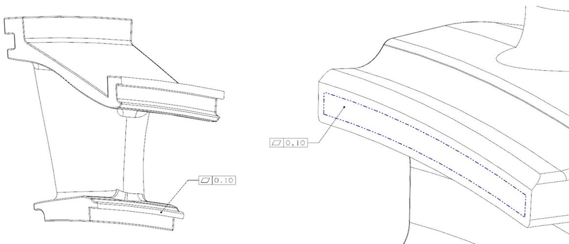
*Fig.5.9. Flatness requirement for a datum placement (0,10 mm). Tight but critical tolerance example. CMM measurement zone on the right picture[38].*
