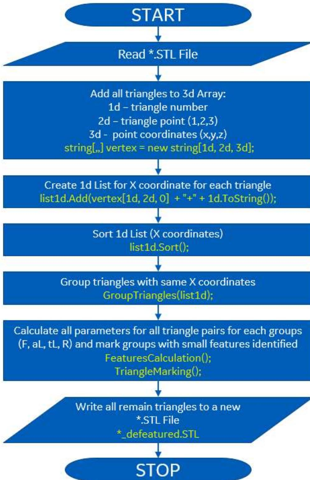
Fig.5.18. Final algorithm coded in C# environment[38].
