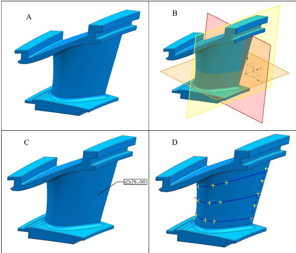
*Fig.4.4. Four levels of MBE definition a) Solid geometry b) Datum System c) PMI definition d) Inspection data*
