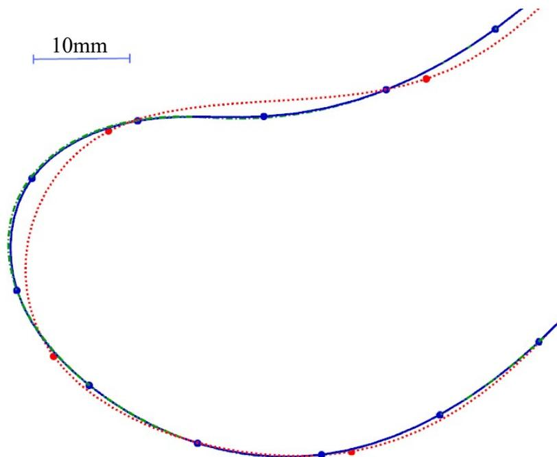
Fig.5.6. Overlay of three B-splines. 10 knots - red – dashed; 25 knots - blue – straight, 104 knots original - green dotted-dashed [39]
