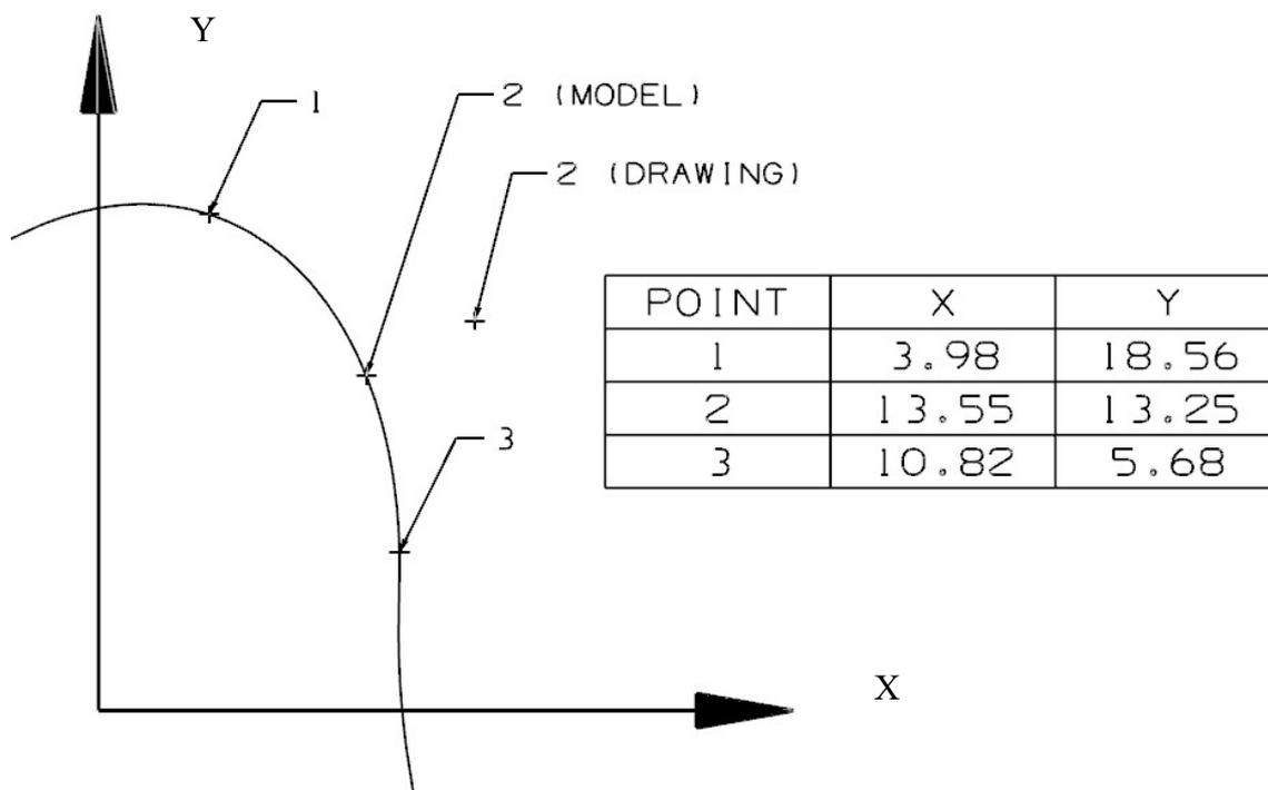
*Fig.1.17. Point definition defined in a 2D drawing is model-independent and can lead to an error.*
