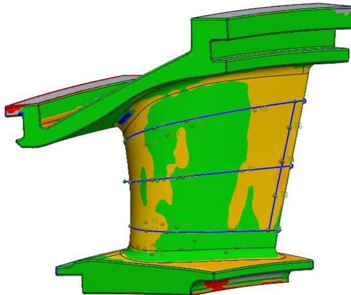
*Fig.1.16. Example of a definition with additional data for inspection inside a neutral format file used for a 3D scan inspection.*
