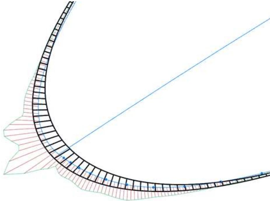
*Fig.1.11. Airfoil leading edge shape (initial example in blue/green/red) adjusted by an external software exceeding CAD capability (in black).*
