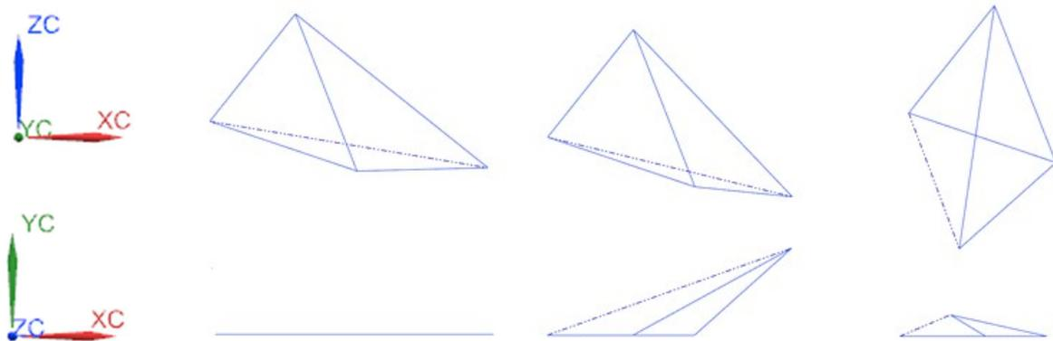
Fig.5.14. Two triangles would lie on a flat surface if the distance between two not shared points (dashed line) reached a local maximum. The smaller distance it has, the more curved surface they represent[38].
