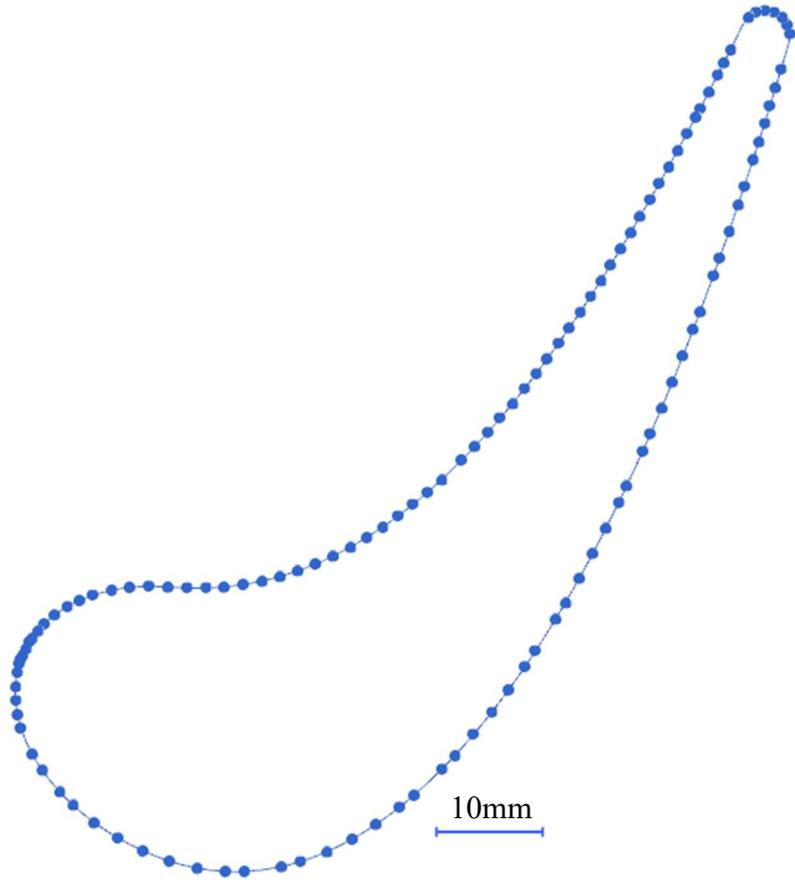
Fig.5.4. Initial control section as a collection of 104 Bezier curves[39]
