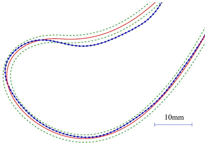
Fig.5.7. Nine hundred ninety-nine points on a B-Spline; blue dot line – deformed part shape exceeding the tolerance zone (green dashed line), red straight line – ideal shape [39].
