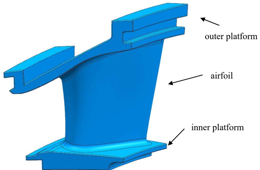
*Fig.1.4. Turbine guide vane example.*
