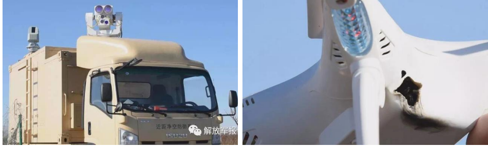
Figure 3. GuoRong Technology based system mounted on trucks (a) capable of civilian drone neutralization (b) [9].
