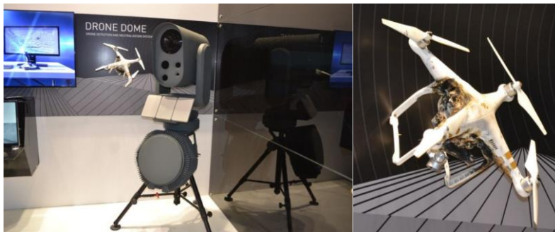
Figure 4. [LEFT] Drone Dome-L system developed by Israeli company Rafael. [RIGHT] Commercially-available drone destroyed by the system [6].
