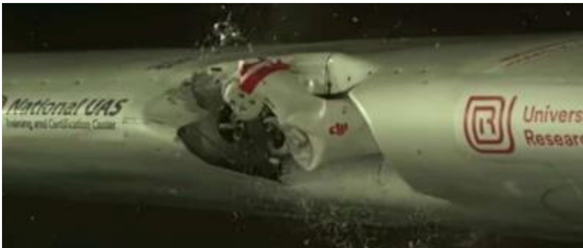
Figure 1. Dayton University based research - drone impact on airplane wing [4].
