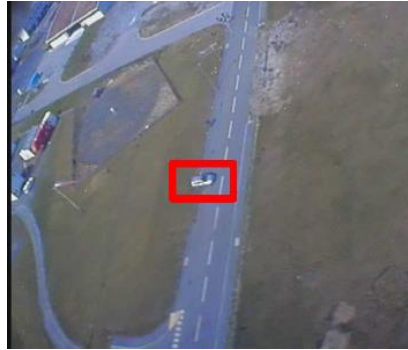
Figure 29. Example of Haar Cascade utilization on UAVs, in this instance for vehicle detection [195].
