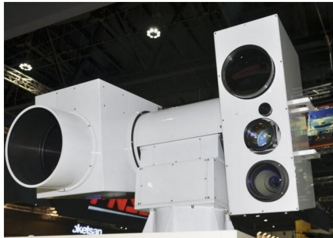
Figure 2. LASS system laser (on the left) and detection and data acquisition system (on the right) [8].
