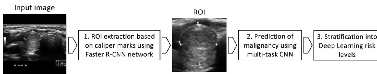
Figure 2: Flowchart of the three main processing stages of our deep learning algorithm. CNN = convolutional neural network, R-CNN = Region-based CNN, ROI = region of interest.
