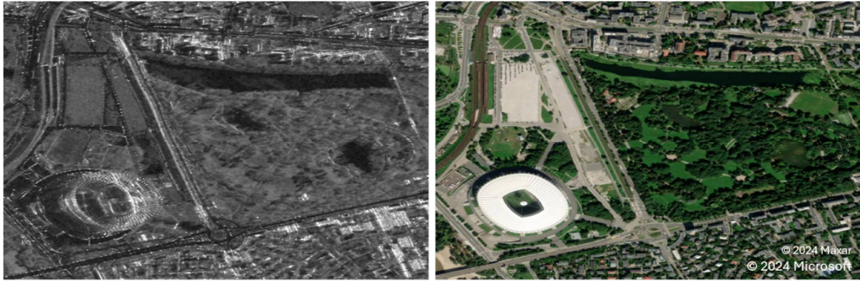
Figure 2.6 Log Intensity SAR image of the National Stadium in Warsaw, Poland, captured by ICEYE in 2023 (left) [8]. Optical images from Bing Maps Satellite Imagery (right) [28].
