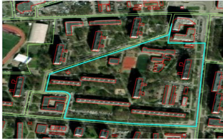
Figure 7.14. Aerial orthophoto of Warsaw from ESRI World Imagery [197] and a selected UA polygon (in cyan) labeled as Continuous Urban Fabric (>80%). Highlighted in red are building footprints from BDOT10k dataset. In this example, there is roughly only 30% occupied of artificial surfaces.
