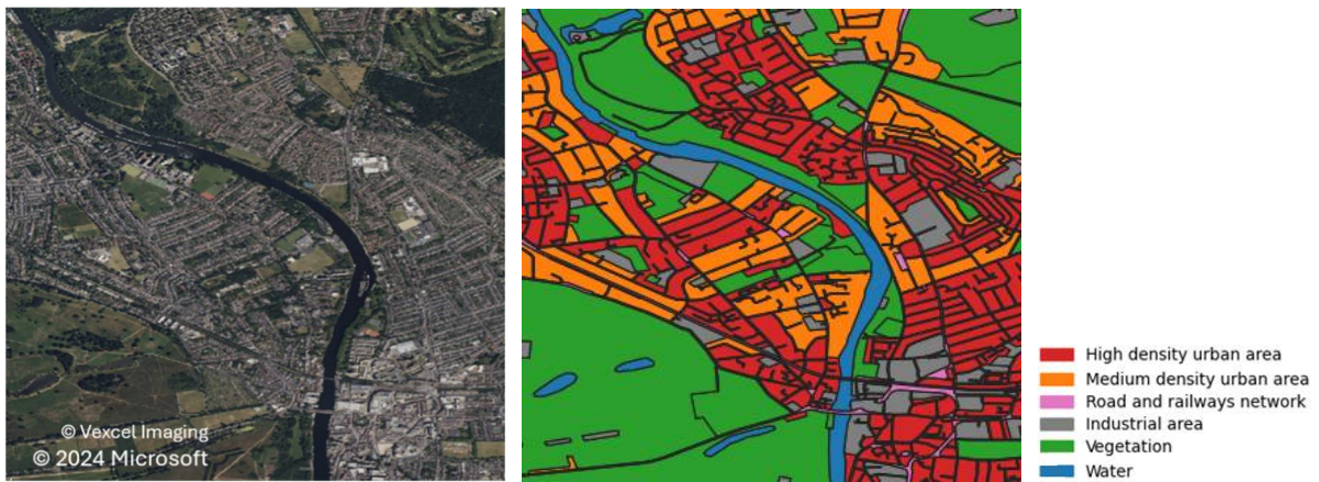
Figure 7.2 A snippet from the scene in London for comparing SAR features. Left: optical image from Bing Maps Satellite Imagery [28]. Right: corresponding UA labels [188].
