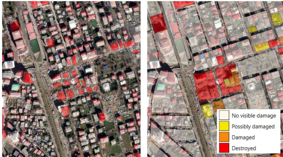
Figure 4.3 Example of different unit analysis: (left) Building unit in binary class damage system of intact buildings and destroyed buildings. (right) Block unit in four class damage system. Optical images from Maxar [5].
