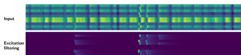
Figure 4. Post-processing of the similarity scores generated by the pre-trained embedder. The first matrix, denoted as input , shows an example of raw distances between the embeddings of keyword patterns and recording fragments. Each row corresponds to a single pattern, while each column represents a single time step. Brighter colours indicate smaller distances (closer matches). The second matrix shows the same values after row-wise standardisation and filtering through the exciter module.
