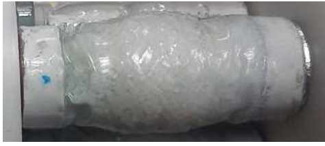
Fig. 4. VPP damper filled with polystyrene
