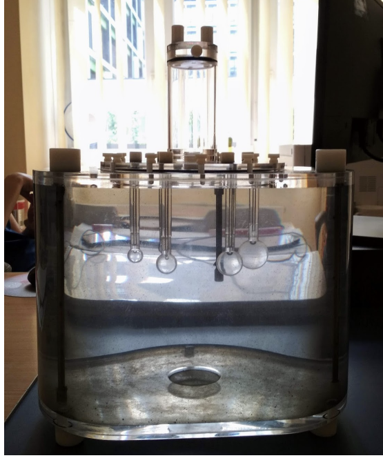
FIGURE 5.5: Picture of the PET-CT phantom BIODEX MEDICAL SYSTEMS available at the Nuclear Medicine Department of the Medical University of Warsaw.
