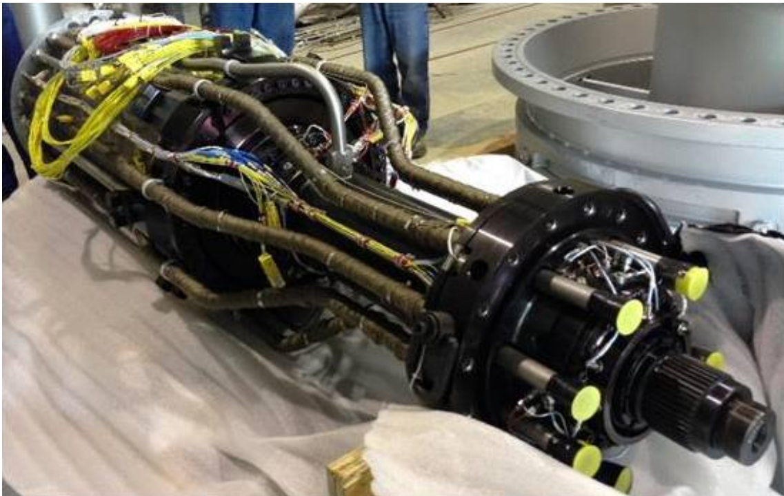
Figure 68 – bearing cartridge used during the GE9X tests (photo courtesy of Polonia Aero)
