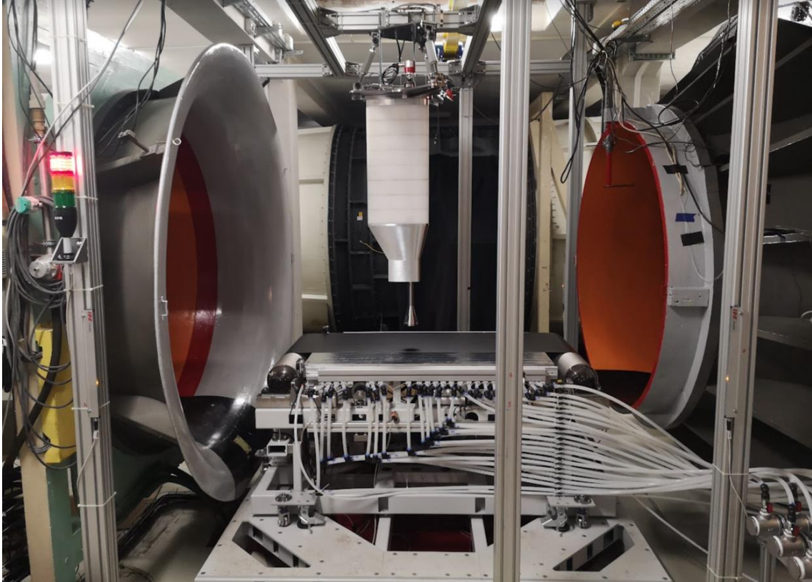
Figure 69 – the moving ground system in the wind tunnel (photo courtesy of Łukasiewicz Research Network – Institute of Aviation)
